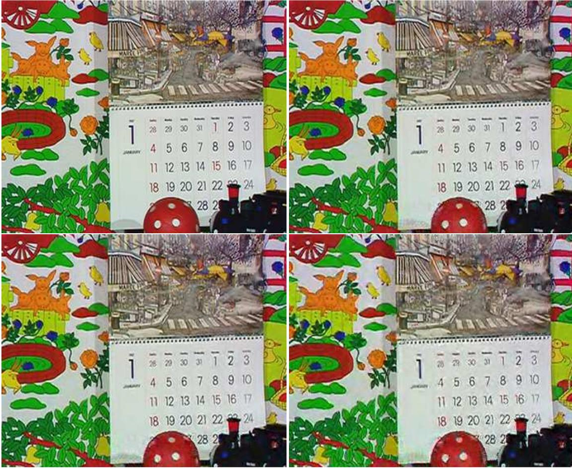
Fig. 12. Comparison of reconstructed frames coded at 586 kbps with different accurate MCTFs: (a) top left: original frame, (b) top right:  $\frac{1}{4}$ -pixel accuracy, Y-PSNR = 28.4 dB, (c) bottom left:  $\frac{1}{2}$ -pixel accuracy, Y-PSNR = 27.3 dB, (d) bottom right: integer-pixel accuracy, Y-PSNR = 25.2 dB.
