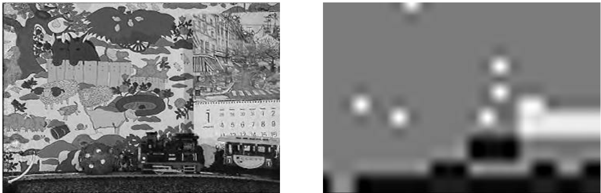
Figure 5: Left: average loss 9.4 %, average burst length = 2. Right: average loss 9.4 %, average burst length = 5.
