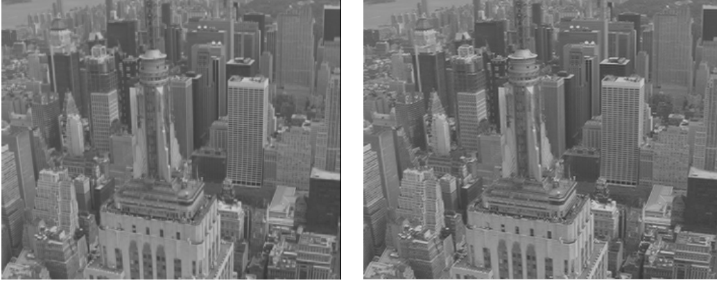
Figure 4. Left: reconstructed low resolution frame after scaling HL, LH and HH bands of Subband low resolution frame with structure one, right: reconstructed low resolution frame after scaling the 12 small bands of Subband low resolution frame using the set of \tilde{\alpha} in Table 2. Both figures are Y component only.
