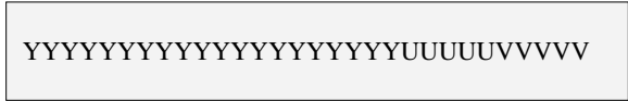
Figure 7: Initial internal structure of LIP and LIS, assuming the U and V planes are one-fourth the size of the Y plane.
