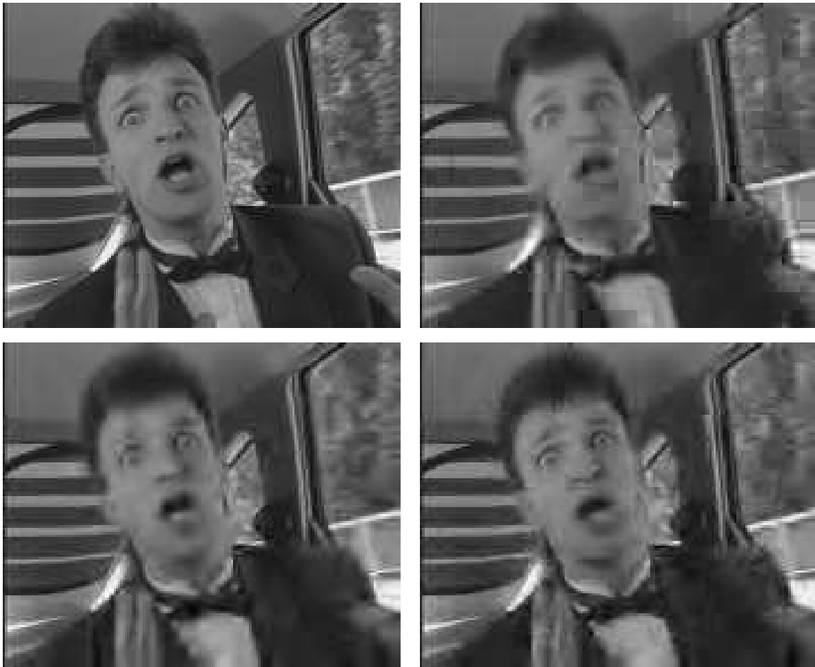
Figure 13: The same reconstructed frames at 30 kbps and 10 f/s (a)Top-left: original “Carphone” frame 198 (b)Top-right: H.263 (c)Bottom-left: 3D SPIHT (d)Bottom-right: MC 3D SPIHT.
