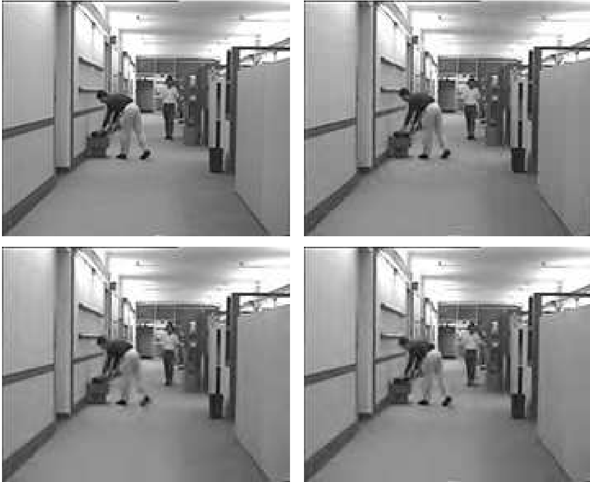
Figure 15: The same reconstructed frames at 30 kbps and 10 f/s (a)Top-left: original “Hall Monitor” frame 123 (b)Top-right: H.263 (c)Bottom-left: 3D SPIHT (d)Bottom-right: MC 3D SPIHT.
