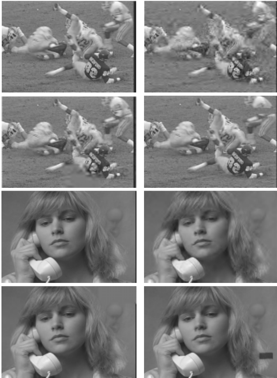
Fig. 19. (a) Top-left : 352 \times 240 original “Football” sequence (frame15), (b) Top-right : 352 \times 240 “Football” reconstruction using normal 3-D SPIHT/FEC with BER = 0.01. PSNR = 24.41dB, (c) Second row-left : 352 \times 240 “Football” reconstruction (frame15) using STTP SPIHT( P=16 )/RCPC with BER = 0.01. PSNR = 29.35dB, (d) Second row-right : MPEG-2/RCPC with BER = 0.01, PSNR = 27.45 dB, (e) Third row-left : 352 \times 240 original “Susie” sequence (frame29), (f) Third row-right : 352 \times 240 “Susie” reconstruction using normal 3-D SPIHT/RCPC with BER = 0.01. PSNR = 32.68 dB, (g) Bottom-left : 352 \times 240 “Susie” reconstruction (frame29) using STTP-SPIHT( n=16 )/RCPC with BER = 0.01. PSNR = 38.53dB, (h) Bottom-right : MPEG-2/RCPC with BER = 0.01, PSNR = 32.84 dB. Total transmission rate is set to 2.53 Mbps.
