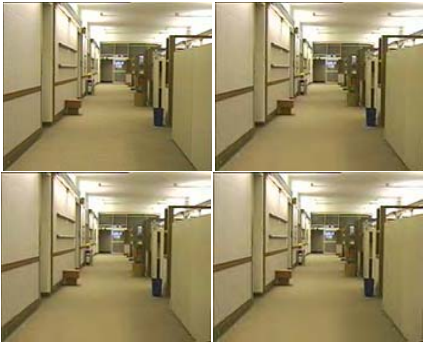
Fig. 13. Reconstructions of first frame of Hall Monitor sequence compressed to 28,500 bits: Original (top left), CSPECK (top right), SPIHT (bottom left), and JPEG2000 (bottom right).
