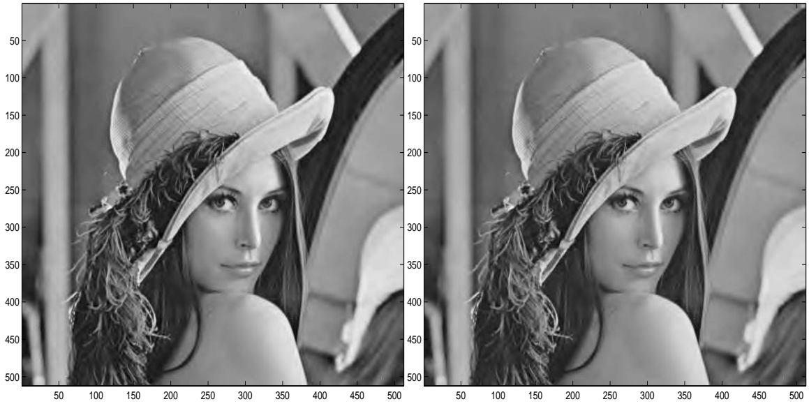
Figure 9: Lena image restored after SPIHT compression at 0.25 bpp rate. From left to right: our 7 tap filter result, 9/7 filter result
