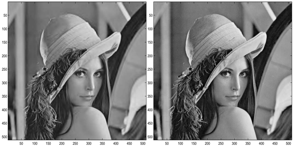
Figure 10: From left to right: Lena image restored after SPIHT compression at 0.25 bpp rate, under 10/18 filter, Original Lena image
