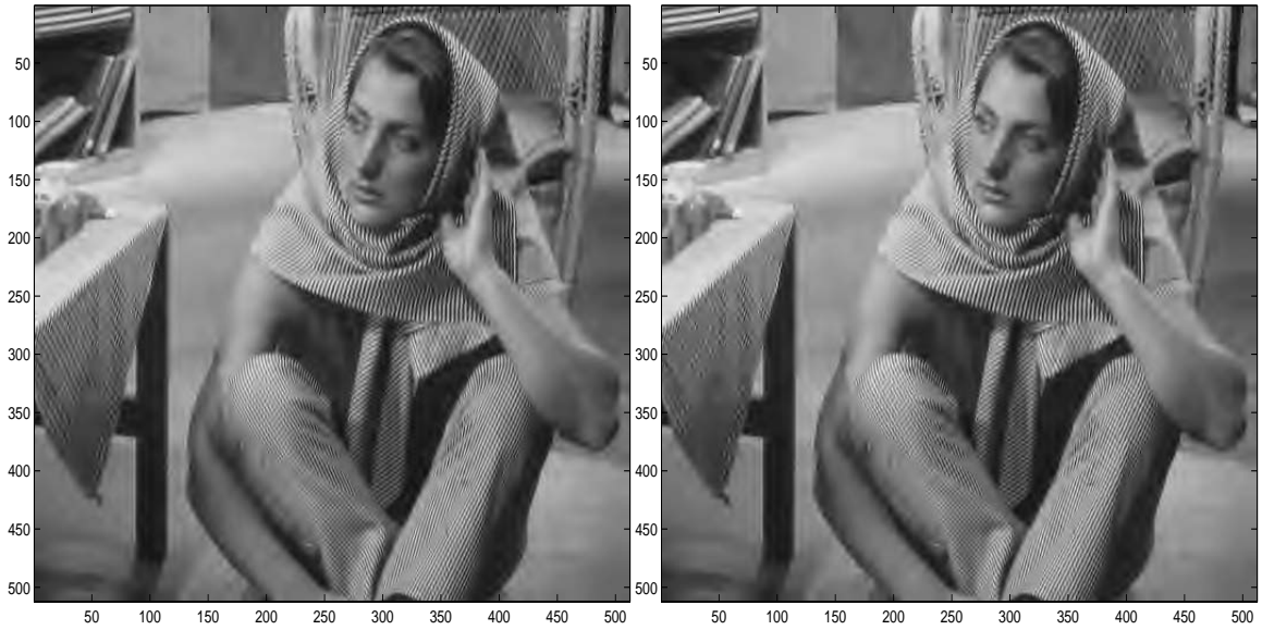
Figure 11: Barbara image restored after SPIHT compression at 0.25 bpp rate. From left to right: our 7 tap filter result, 9/7 filter result
