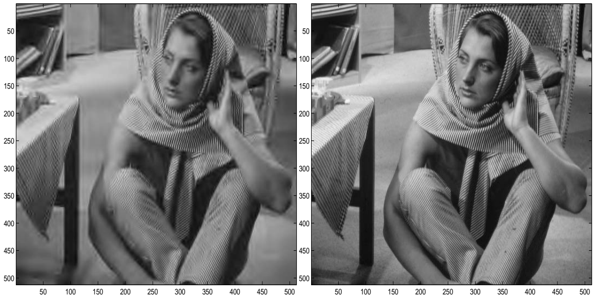
Figure 12: From left to right: Barbara image restored after SPIHT compression at 0.25 bpp rate, under 10/18 filter, Original Barbara image
