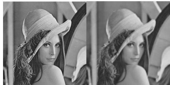
Figure 5 Left: Original Lenna512 Right: Reconstructed Lenna512 after 9 passes (MSE = 17.65, Original SPIHT Rate = 0.3498, SPIHT with all four modifications Rate = 0.3447)
