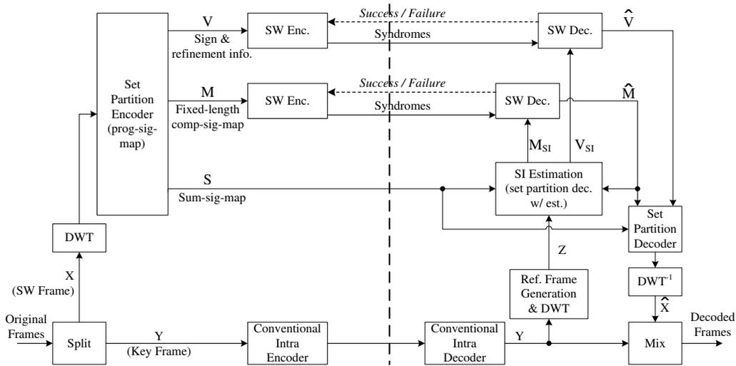
Figure 1: Block diagram of the proposed DVC system based on SPC with prog-sig-map.
